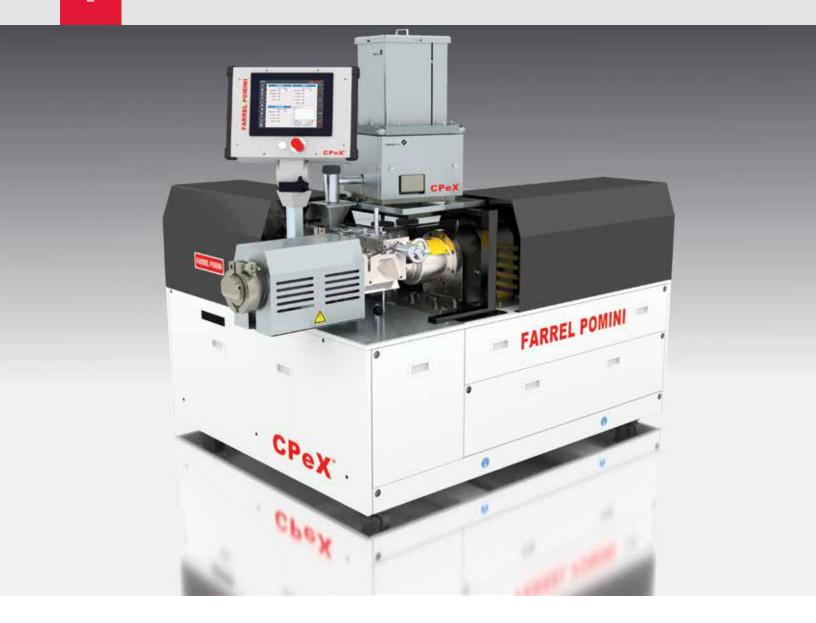
The CPeX® is the Laboratory Compact Processor utilizing the unique and proven FARREL POMINI continuous mixer technology in a size suitable for testing and development. The CPeX®'s design allows compounders to conduct laboratory scale product development trials, extend product application portfolios, expedite time to market and reduce development costs.
